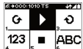
If the standard acknowledgement view is activated, the corresponding function field is displayed inverted while a function key is pressed. The transmission data used and the address used from the assigned definition are displayed in the header during transmission.
