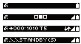
For certain transmitted data, the addition T1, ..., T8 is displayed. For SVS products, this suffix is often used as the name of the bit combination.
