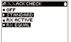
The currently selected menu item is inverted and displayed with a triangle. If it is a menu in which a setting can be made, the current setting is displayed inverted with a square. In this case, the **✓** key can be used to accept the current selection and then switch to the higher-level menu. The **X** key can be used to switch to the higher-level menu without accepting the selection.
