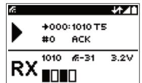
The upper half gives information about outgoing transmissions. The set characters are displayed on the left in accordance with the assigned definition. Next to this are the address used, the data sent, the number of transmission attempts per message and the current acknowledgement setting.
