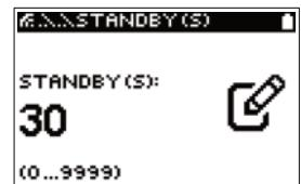
The footer may show the allowed value range. If the minimum and maximum have the same number of digits (e.g. 000 ... 999), this is also an indication of a fixed input length. Otherwise (e.g. 0 ... 9999) the length of the input is variable.
