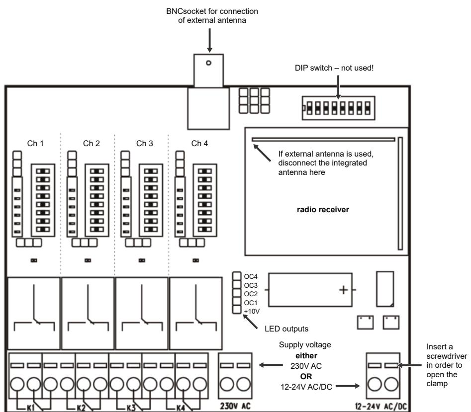
Each learn mode returns to normal receiving mode if a valid signal has been received, or if the LEARN/ERASE button is pressed again, or if the learn- and erase mode is already active more than 30s. The LED next to the LEARN/ERASE button only lights, if the radio receiver DIP switch 6 is "ON".
