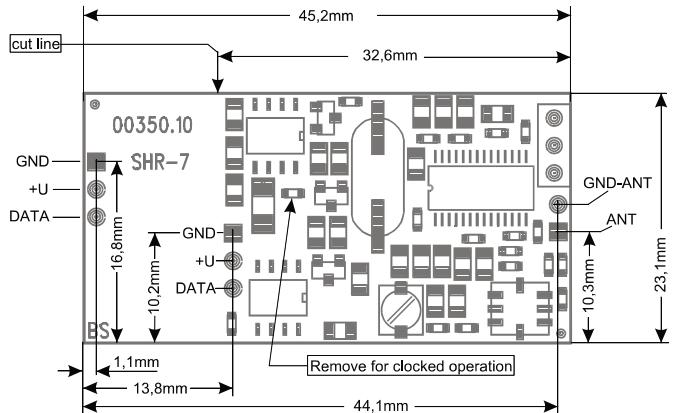
Data Output: Transistor output with 15 kOhm pull-up resistor with +5V internally controlled. The data sequence received from the transmitter at the receiver output is inverted. This needs to be taken into account when processing the data.
