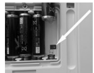
Picture 2: Tune volume of internal loudspeaker
