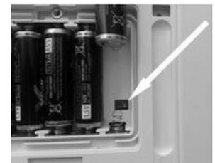
Picture 2: Tune volume of internal loudspeaker
