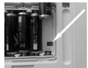
Picture 2: Tune volume of internal loudspeaker
